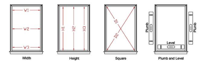
If there is an issue with any of the above, **DO NOT INSTALL** the window and contact your window and door distributor.
